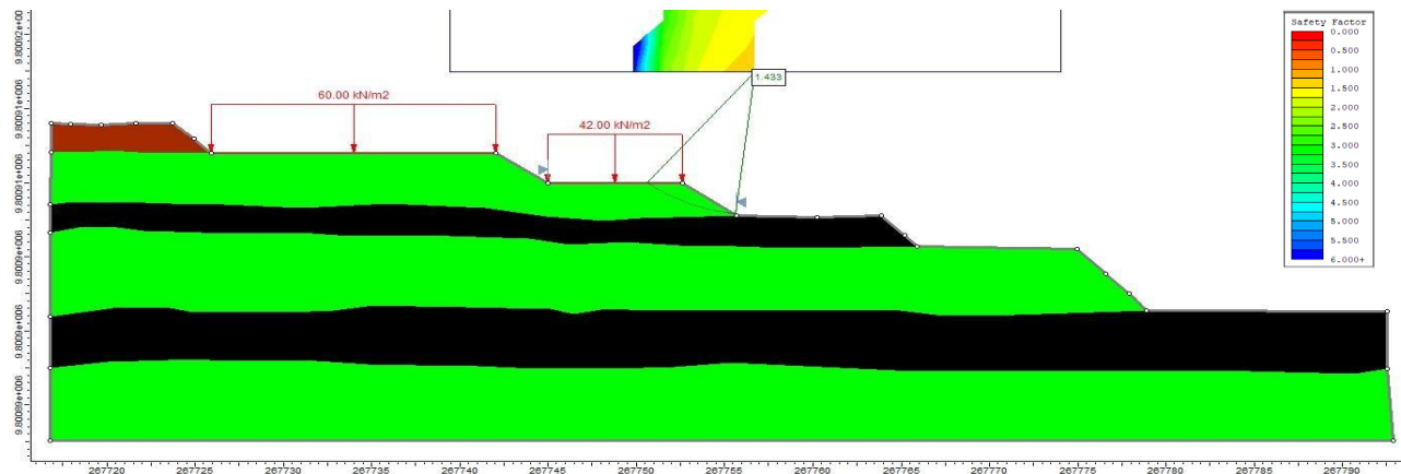
Figure 11. Analysis Results of the Redesign Existing Single Slope on bench 3 Section B-B'
