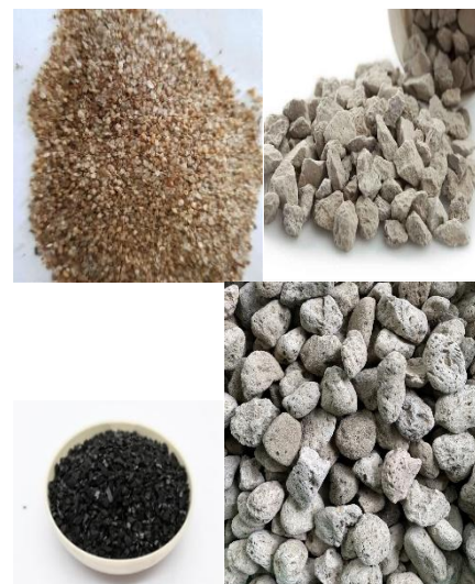
Gambar 2. Media Kontak Scaling Mitigation Reactor
